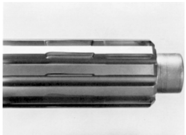
Input spline wear
